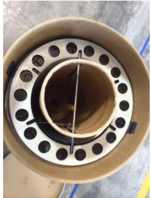
Unfasten the stitching wire end from the center hub of the drum and remove the steel bar and 2 plastic rings. Discard the steel bar and black protector ring. The light colored guide ring will be reused and should not be discarded.
