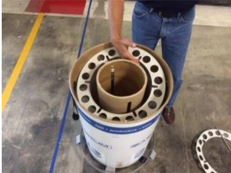
The metal guide basket should be placed with narrow dimension facing down and fitted into the slots of the plastic guide ring.
