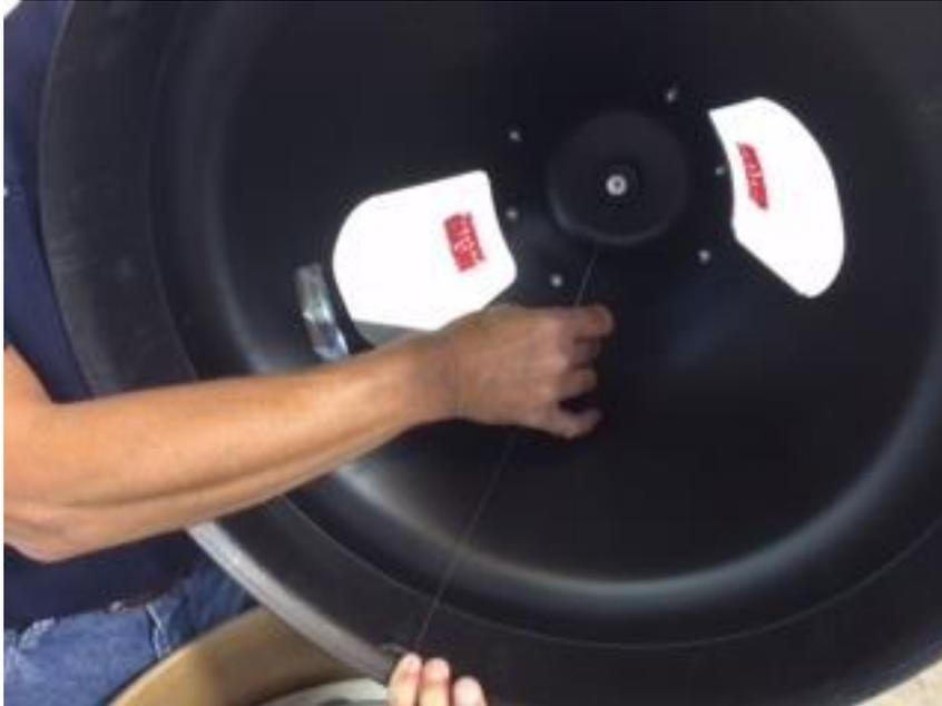
Place drum lid on drum and feed wire through the supplied conduit tube.
