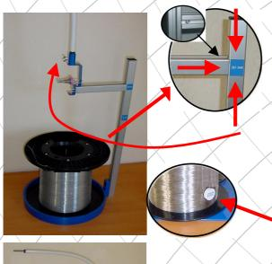
First bring the **tension adjustment arm in position** as shown on the base unit mark. For the adjustment use an allen wrench 2,5mm. The **allen screw** is at the **backside** of the arm showing in detailed picture.
