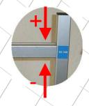
Note: Lifting or reducing the high of the adjustment arm decreases or increases the tension of the stitching wire.
